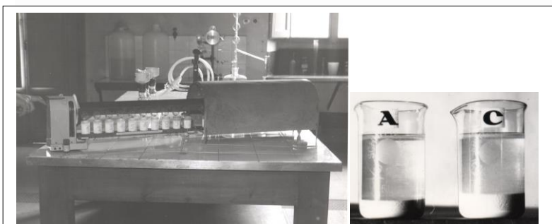
Fig. 2 - Execution of test P: the precipitation of BiOCl is carried out in 2 sets of 10 beakers each, one in open air and the other under a thin copper screen (see text for details).
